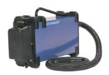
Fume Eliminator 840/841 is a small, lightweight, portable extraction unit designed to be carried to the working area. Connected to a welding torch or to an extraction nozzle, the FE 840/841 unit extracts the fume directly at source. FE 840 has a manual start/stop function. FE841 has an automatic start/stop function which starts the unit as soon as the welding begins. It also includes an indicator for filter exchange.
