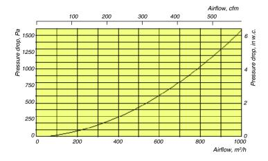
Pressure drop valid for 6 and 7 m track with 5 m hose, Ø 125 mm, and HB 600LL nozzle.
