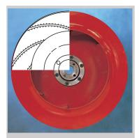
The rounded impeller is used for transport of clean air and air with a small amount of fine dust, such as welding smoke, oil mists or exhaust gas. This impeller has an efficiency of up to 85%.
