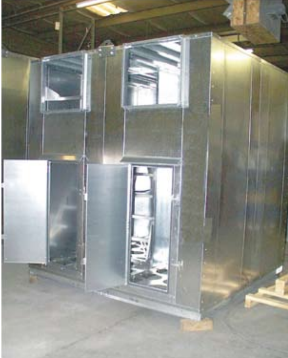
Baghouse under construction
