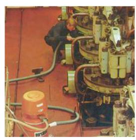
The vacuum units can be supplied with a wide range of capacities to meet customer requirements. Tank capacities can be either 67 or 200 litres, or silo systems can be supplied.
