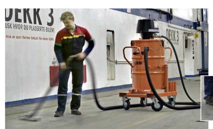
Nederman is a world-leading manufacturer of vacuum power products. Its Norclean Line of compressed-air powered ejector vacuum cleaners is designed for collection of virtually anything that can flow through a hose, whether it is liquid, dust or granules.
